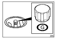
Check the integrity of gaskets (indicated with [G] in the figure) and substitute those that are deteriorated.
